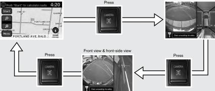
When the shift lever is in the R (REVERSE) position and the CAMERA button of is pressed, the following views will display in order:
