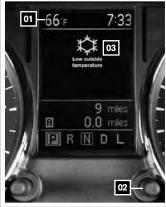
To stop the outside temperature display from blinking, stop the vehicle in a safe place and move the shift lever to the (P) PARK position. Perform the following procedure:
