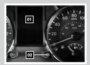
■ If the cap is not properly tightened, the Malfunction Indicator Light () may illuminate.
