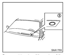
Be sure not to put anything on top of the photo sensor (1) located on the top of the instrument panel. The photo sensor controls the autolight; if it is covered, the photo sensor reacts as if it is dark and the headlights will illuminate.
