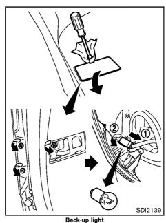
Open the lift gate to remove the back-up light assembly. One screw is located behind the cover on the lift gate.
