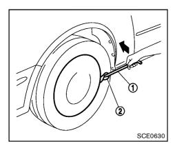
Removing wheel cover (if so equipped)
