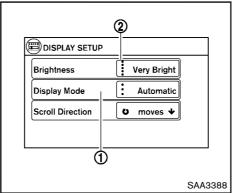
Other items are adjusted by selecting one of a set number of conditions. For example, the Display Mode can be set to "Automatic", "Day" or "Night". To adjust this type of item, touch the item (1). The item will cycle through the available settings and the red indicator lights to the left of the setting condition (2) will come on or turn off accordingly.
