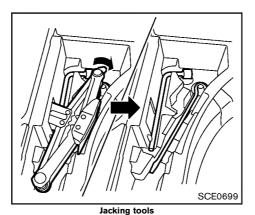
Remove the jacking tools and the spare tire.
