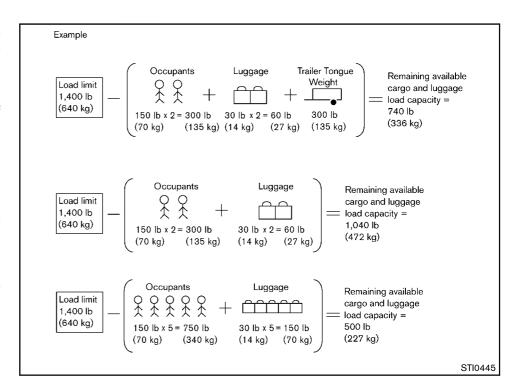
Steps for determining correct load limit
