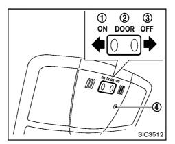
The map light control switch has three positions: ON (1), DOOR (2) and OFF (3).
