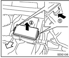
Push the tabs ① and pull out the filter element ②.
