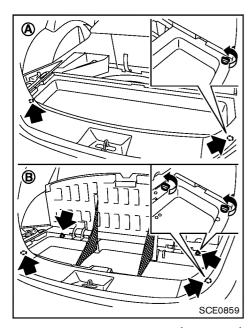
5. Remove the luggage floor box (Type A or B) by turning the clips counterclockwise.
