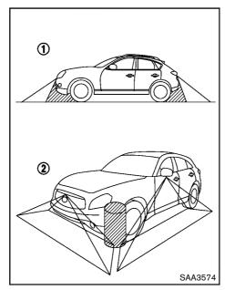
There are some areas where the system will not detect objects. When in the front or the rear view display, an object below the bumper or on the ground may not be detected ①. When in the bird's-eye view, a tall object near the seam of the camera detecting areas will not appear in the monitor ②.
