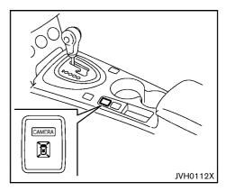
The CAMERA button is located on the center console.
