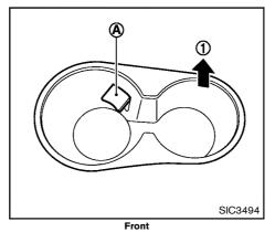
The flap (A) will be folded down when inserting a large container.
