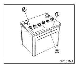
Check the fluid level in each cell. (Remove the battery cover if it is necessary.) It should be between the UPPER LEVEL (1) and LOWER LEVEL (2) lines.
