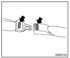
The center seat belt buckle and the tongue are identified by the CENTER mark. The center seat belt tongue can be fastened only into the center seat belt buckle.
