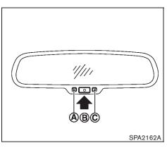
When the system is turned on, the indicator light (A) will illuminate and excessive glare from the headlights of the vehicle behind you will be reduced.
