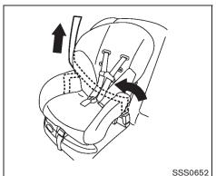
Front-facing — step 5 5. Allow the seat belt to retract. Pull up on the shoulder belt to remove any slack in the belt.
