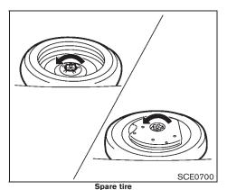
Spare tire: Turn the clamp to remove the tire.
