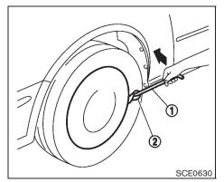
Removing wheel cover (if so equipped)
