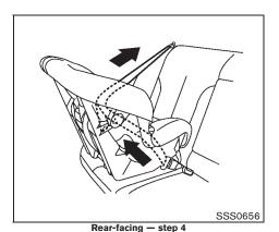
4. Allow the seat belt to retract. Pull up on the shoulder belt to remove any slack in the belt.
