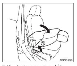
Folding front passenger's seat (if so equipped)
