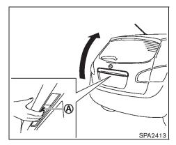
To open the lift gate, unlock it and push the opener switch (A). Pull up the lift gate to open.
