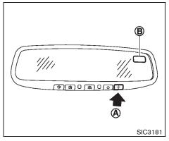
When the ignition switch is turned to the ON position, the compass display (B) will indicate the direction of the vehicle's heading.
