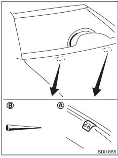
Be careful not to clog the washer nozzle (A). This may cause improper windshield washer operation. If the nozzle is clogged, remove any objects with a needle or small pin (B). Be careful not to damage the nozzle.
