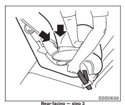
For child restraints that are equipped with webbing-mounted attachments, remove any additional slack from the anchor attachments. Press downward and rearward firmly in the center of the child restraint with your hand to compress the vehicle seat cushion and seatback while tightening the webbing of the anchor attachments.
