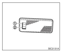
When the switch is in the ON position ①, the light illuminates while the lift gate is opened. When the lift gate is closed, the light will turn off.
