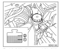
Check the fluid level in the reservoir. If the fluid is below the MIN line (1) or the brake warning light comes on, add Genuine NISSAN Super Heavy Duty Brake Fluid or equivalent DOT 3 fluid up to the MAX line (2). If fluid must be added frequently, the system should be checked by a NISSAN dealer.
