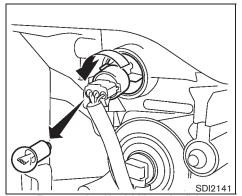
Front turn signal/park/side marker light (Halogen headlight model) Xenon headlight model: See a NISSAN dealer for replacement.
