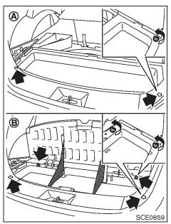
6. Remove the luggage floor box (Type A or B) by turning the clips counterclockwise.
