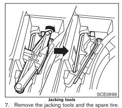
Jacking tools: Remove the jack by turning it, then remove the other tools.
