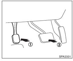
To apply: Fully depress the parking brake pedal **(1)**.
