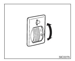
Headlight aiming control (if so equipped) Depending on the number of occupants in the vehicle and the load it is carrying, the headlight axis may be higher than desired. If the vehicle is traveling on a hilly road, the headlights may directly hit the rearview mirror of the vehicle ahead or the windshield of the oncoming vehicle. The light axis can be lowered with the
