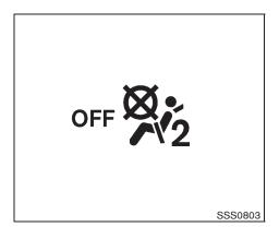
7. If the booster seat is installed in the front passenger seat, turn the ignition switch to the ON position. The front passenger air bag status light of the may not be illuminated depending on the size of the child and the type of booster seat used. (See "Front passenger air bag and status light" later in this section.)
