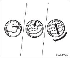
Open or close, and adjust the air flow direction of ventilators as illustrated.
