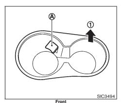
The flap (A) will be folded down when inserting a large container.
