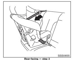
Pull the shoulder belt until the belt is fully extended. At this time, the seat belt retractor is in the Automatic Locking Retractor (ALR) mode (child restraint mode). It reverts to the Emergency Locking Retractor (ELR) mode when the seat belt is fully retracted.
