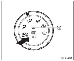
To defog/defrost the rear window glass and outside mirrors (if so equipped), start the engine and push the switch on. The indicator light ① will illuminate. Push the switch again to turn the defroster off.
