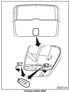
The license plate light bulb can be accessed by removing the cover on the inside of the lift gate.
