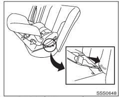
Rear-facing (webbing-mounted) - step 2 2. Secure the child restraint anchor attachments to the LATCH lower anchors. Check to make sure the LATCH attachment is properly attached to the lower anchors.
