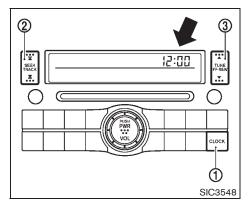
The digital clock (in the audio unit) displays time when the ignition switch is in the ACC or ON position.
