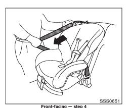
4. Pull the shoulder belt until the belt is fully extended. At this time, the seat belt retractor is in the Automatic Locking Retractor (ALR) mode (child restraint mode). It reverts to the Emergency Locking Retractor (ELR) mode when the seat belt is fully retracted.
