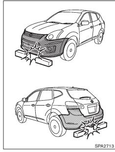
The Krom models have unique front and rear bumpers and exhaust pipes. These parts are close to the ground and may be damaged if they contact objects such as curbs, parking blocks, etc.
