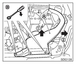
Removing the air duct Remove the air duct (A) if necessary.
