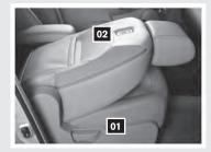
Once the seatback is released, it will enable you to fold the front passenger seatback down over the seat cushion.
